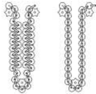
图3 弹链折叠排列与直线排列对比 Fig.3 Comparison of fold arrangement and line arrangement of the ammunition belt
