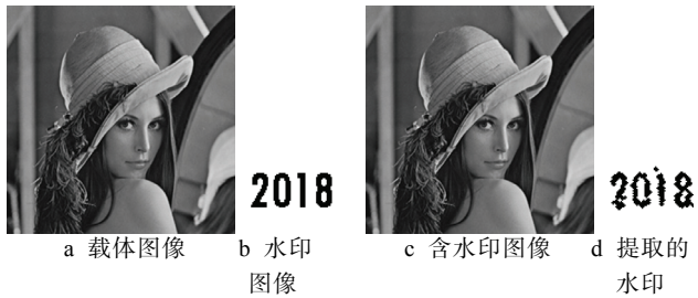
图 8 水印的嵌入和提取 Fig.8 Watermark embedding and extraction
