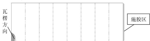
图 1 多边形纸箱侧板平面展开 Fig.1 Plane spreading of the polygonal box side plates
