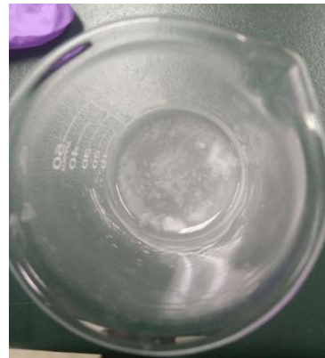
图 1 0.5 g 样品溶于 5 g 水中溶解 2 h 后的结果 Fig.1 Result of 0.5 g sample dissolved to 5 g water after 2 h
