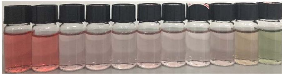
图 1 改性花青素溶液在不同 pH 下的颜色变化 (从左至右 pH 分别为 2~12) Fig.1 Color change of modified anthocyanin solutions at pH 2-12 (from left to right)
