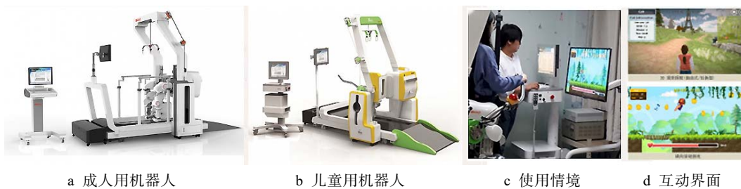
图 9 Walkbot_S 下肢康复机器人及其软件界面 Fig.9 Walkbot_S lower limb rehabilitation robot and software interface
