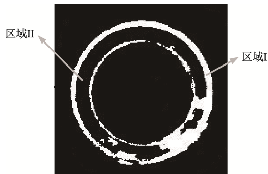
图 3 瓶口缺陷 Fig.3 Bottle mouth defect
