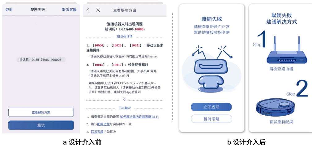
图 8 家用扫地机器人故障报错移动界面设计前后对比 Fig.8 Comparison of mobile interface design before and after fault report of home robot vacuum
