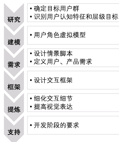
图 1 目标导向设计方法的基本步骤 Fig.1 Basic steps of Goal-oriented design method
