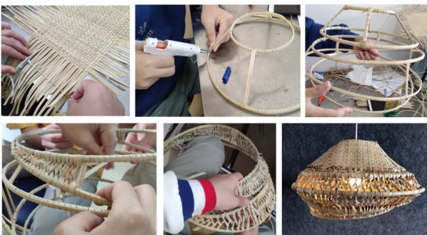
图6 葵编几何灯具的制作过程 Fig.6 The production process of the palm leaf knitted geometric lamp
