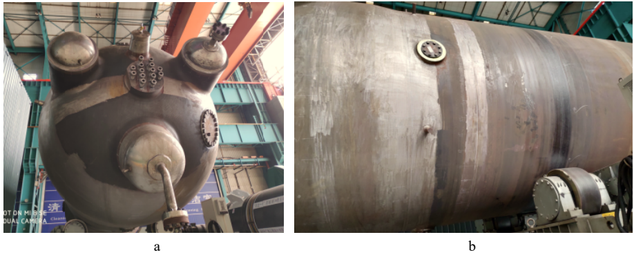
图 4 核一级设备拆开包装后的外观状态 Fig.4 Appearance status of nuclear first-class equipment after unpacking
