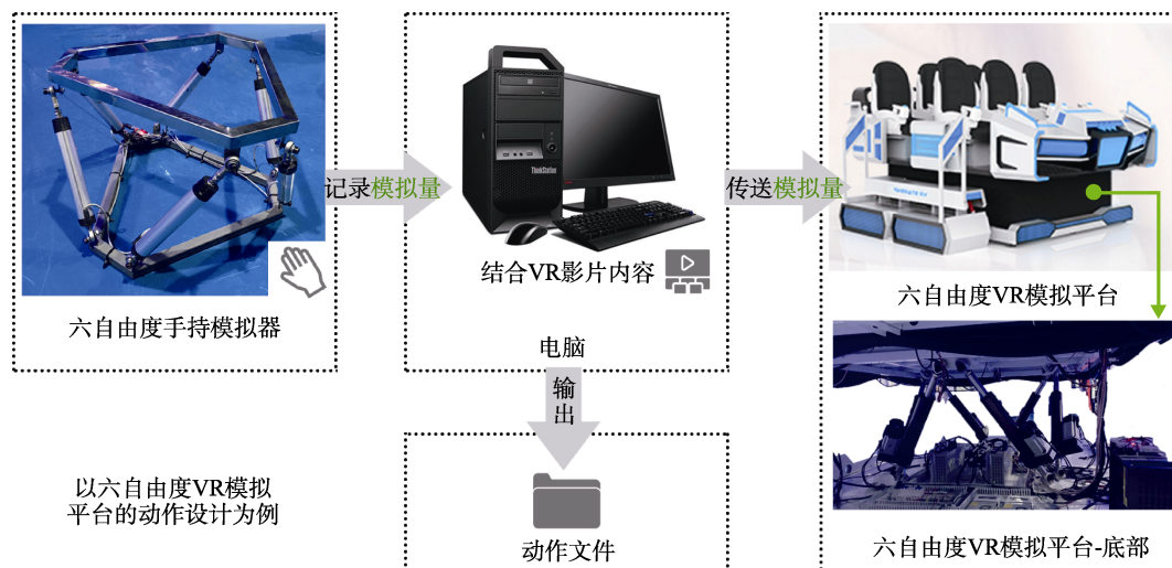
图2 以六自由度VR模拟平台动作设计为例 Fig.2 Take the motion design of 6-DOF VR simulation platform as an example
