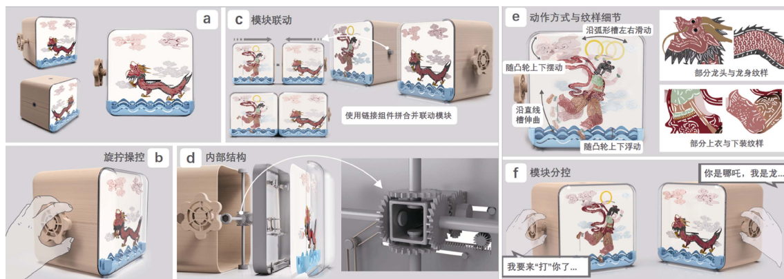
图5 桌面化小型皮影游戏产品设计方案及分析说明 Fig.5 Desktop small shadow puppet game product design plan and analysis description
