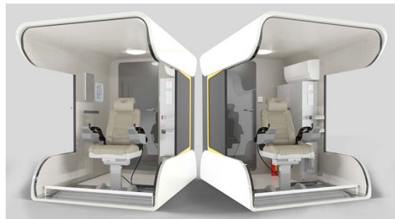
图16 塔机驾驶室空间布局优化设计 Fig.16 Optimized spatial layout design of tower crane cab
