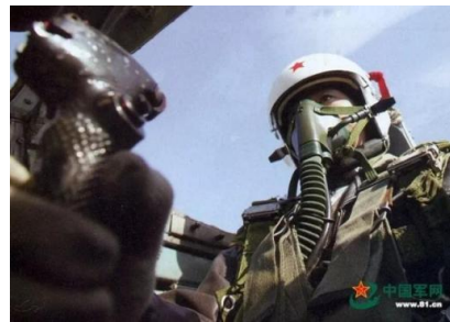
图5 穿着高空代偿服的飞行员 Fig.5 A pilot wearing a partial pressure suit
