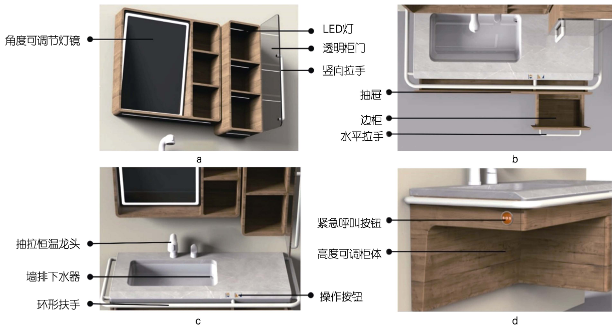
图 3 适老浴室柜细节展示 Fig.3 Details of the bathroom cabinet suitable for the elderly
