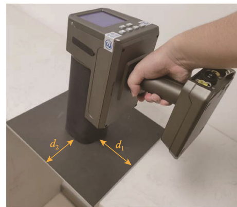
图11 手持测量仪探头与涂层边缘位置关系 Fig.11 Position relationship between handheld measuring instrument probe and coating edge
