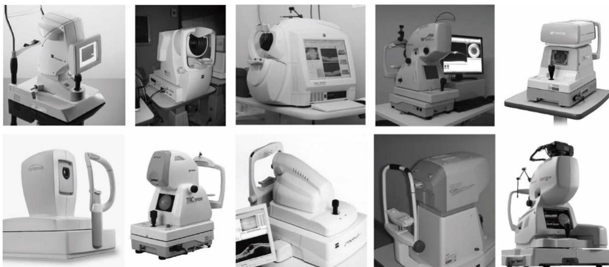
图 5 OTC 仪器的 10 种整体造型设计 Fig.5 10 types types of overall design for OTC instruments
