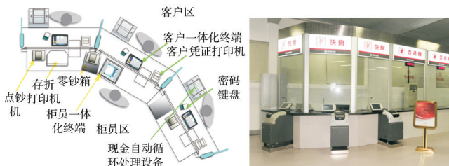
图5 “一对三”服务布置设计 Fig.5 "One to Three" service layout design
