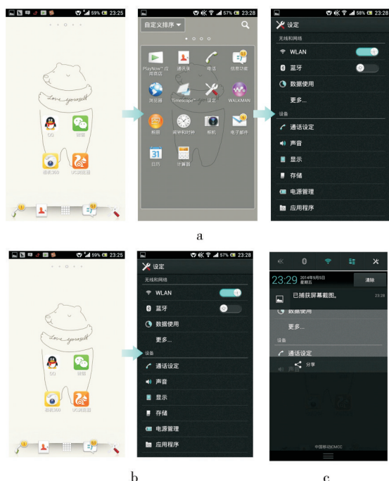
图3 Android4.1.2开启/关闭WIFI的操作路径 Fig.3 Operation pathway to on/off WIFI of Android4.1.2
