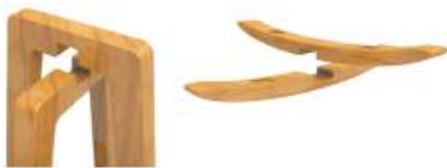
图6 儿童摇摇椅的榫卯结构 Fig.6 The tenon structure of children rocking chair
