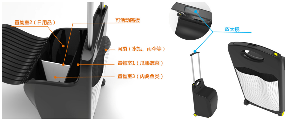
图 5 老人购物车设计 Fig.5 Shopping cart design for the elderly
