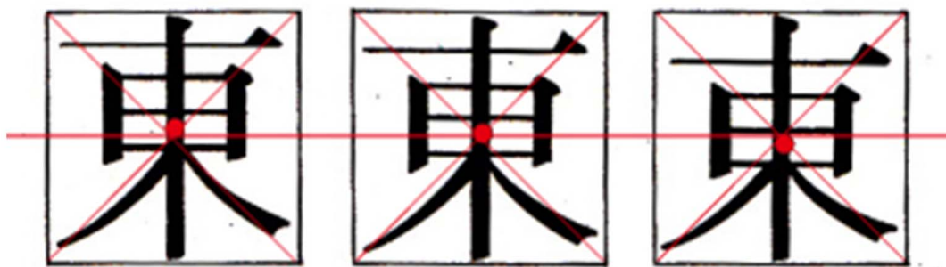
图 5 重心位置设计不同引起字体风格的变化 Fig.5 Variation of font style caused by difference of designed barycenter position
