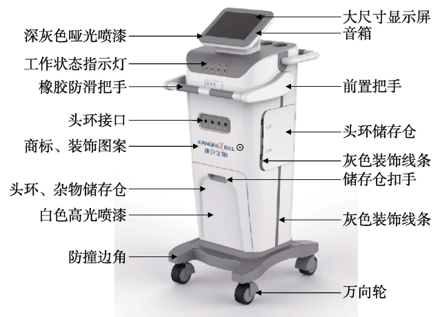
图5 经颅治疗仪主体造型 Fig.5 Main body modeling of transcranial electromagnetic therapy device
