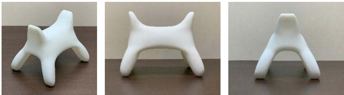
图6 3D 打印儿童家居椅模型输出 Fig.6 Output of 3D printed child home chair model
