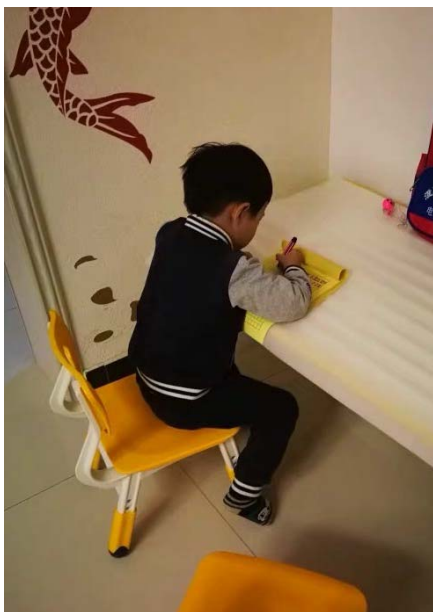
图 10 错误的家具尺寸迫使学生抬起肘部及肩膀并弯腰 Fig.10 Wrong furniture dimensions force students to lift their arms and hunch their shoulders
