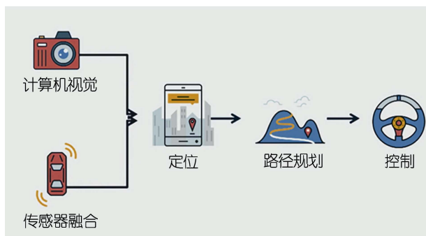
图1 自动驾驶系统的5个核心部分 [11] Fig.1 Five core parts of an autonomous driving system
