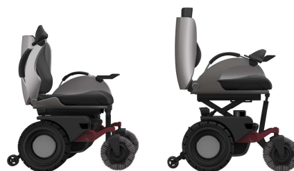
图9 智能轮椅的入座方式示意图 Fig.9 Schematic diagram of the seating method of a smart wheelchair
