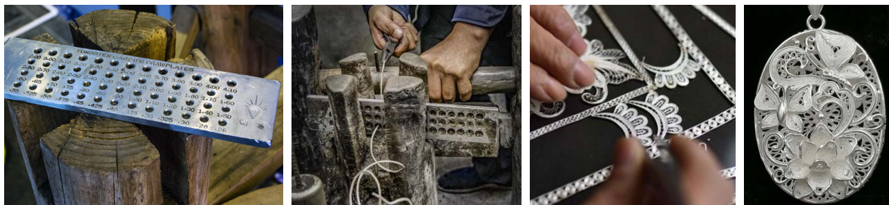
图 4 花丝模具、拉丝填丝过程及银饰成品 Fig.4 Filament mold, drawing and filling process and silver jewelry product
