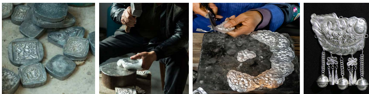
图 3 压模模具、压模过程及银饰成品 Fig.3 Stamping die, stamping process and silver jewelry product
