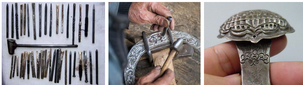
图 6 篆刻工具、篆刻过程及银饰成品 Fig.6 Chisel carving tool, chisel carving process and silver jewelry product
