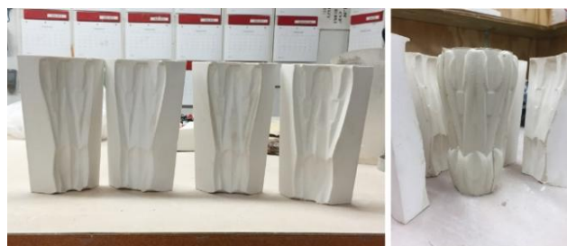
图 8 使用注浆工艺制得的跑车水杯泥坯 Fig.8 Clay of creative car cup made from precise plaster mold
